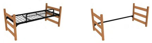
In the above pictures, note that the steel bed spring can be inserted into the posts at residential height or at a higher height. The higher height will allow your items to be placed under the bed for space saving. Note that the spring has two hooks on each end that insert over the steel rods embedded in the wood end (picture below).
